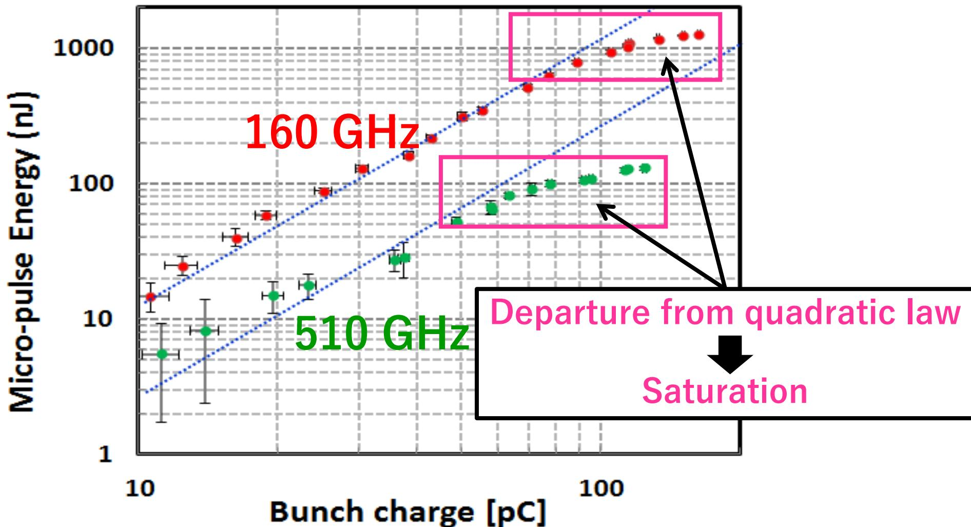
Since the low energy electron beam, space charge effect makes electron bunch length long at the high charge condition. → **Saturation of THz-CUR**
